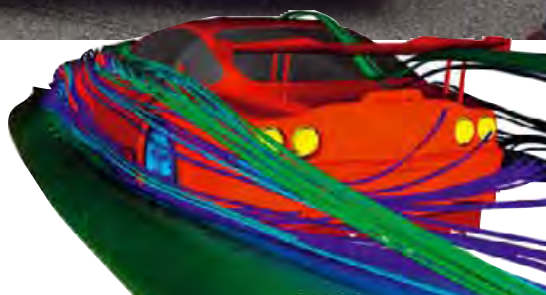
Right – figure 13: the disturbance caused by a mirror can travel well downstream though, as CFD streamlines of a Ferrari 550 show (Advantage CFD)
