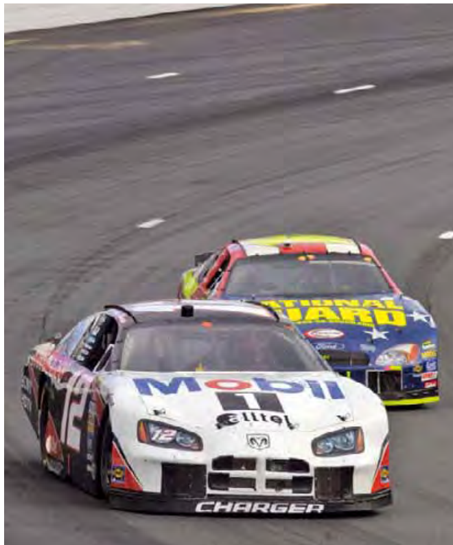
Large left percentage also tightens a car during entry and loosens it in exit (LAT)
